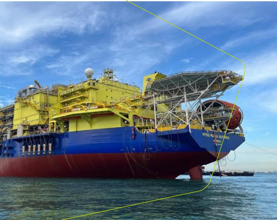
In addition, FPSO Maria Quitéria left the shipyard in May 2024. This platform will operate in the Jubarte field, located in Campos Basin pre-salt on the coast of Espírito Santo, and has advanced carbonization technologies, such as the combined cycle in power generation and the Gas Recovery Unit - FGRU (closed flare). Its production capacity is 100 Mbpd of oil and 5 million m<sup>3</sup>/d of natural gas.
